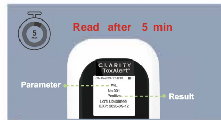
The Reader will automatically display the result after 5 minutes countdown.
