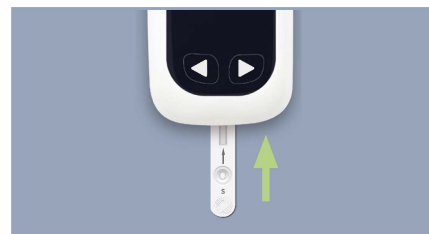
Please ensure that orientation of the Test Device is as shown in the image above.
